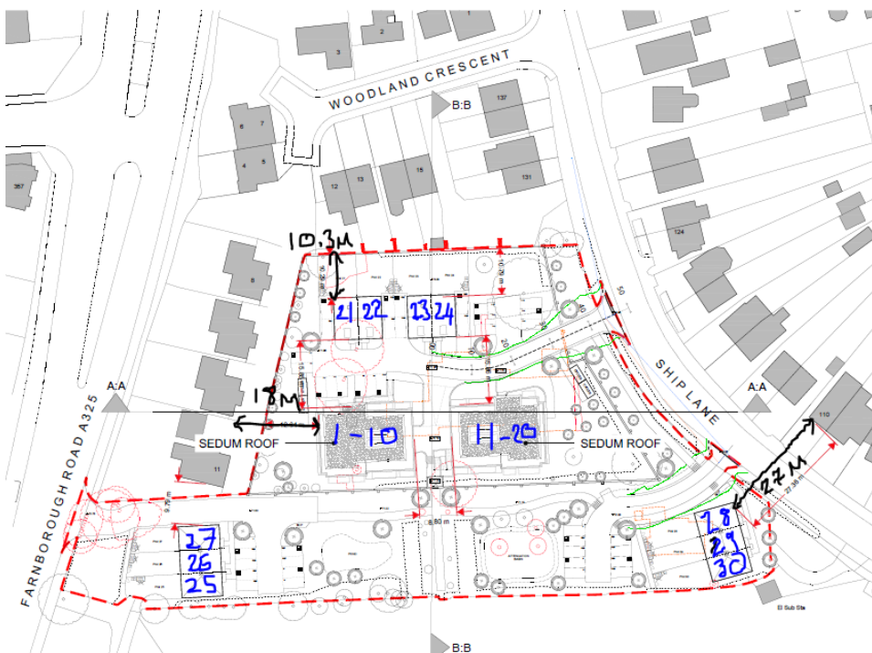
Figure 4: distance separation between units.
